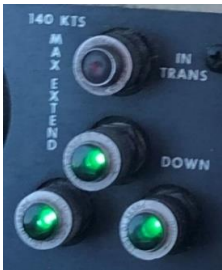
The landing gear switch and landing gear indication system in a Beechcraft Duchess Be-76 aircraft. Note the 'Gear in Transit' light.
