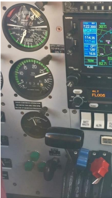
Above we see the levers and MP/RPM readings during take-off in an Arrow III. Note the Fuel Flow
