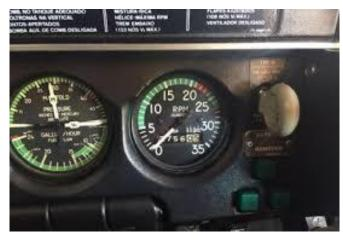
On the ground, with the engine shut down, the RPM will be reading zero, fairly obviously, and the Manifold Pressure gauge will be reading atmospheric pressure in inches of mercury (Usually about 29-31" at sea level but decreases by 1" per 1000' as you gain altitude or elevation).
