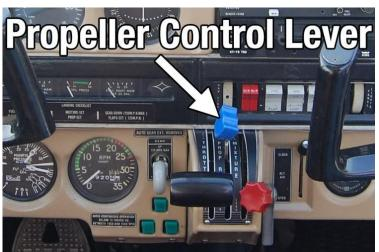
Here, on the left, is the throttle quadrant for a Piper Arrow, showing the new Propeller Control Lever or RPM lever.
