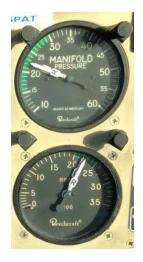
← A twin engined aeroplane set at 22 squared in the cruise
