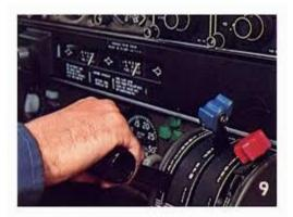
RPM lever should be fully forward when you enter the aircraft.
