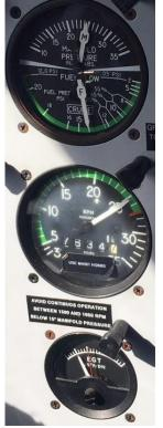
Above we see the levers and MP/RPM readings during take-off in an Arrow III. Note the Fuel Flow
